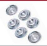
1/4" angular seat rupture discs are designed to be used with the safety head assemblies that are show above. Minimum rupture disc pressure ratings should be at least 110% of system operating pressure. The standard material is Inconel. The pressure ranges indicated in the table below are at room temperature (72°F). Other materials and pressure ranges are available upon request.
