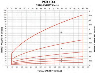
Note: Minimum impact velocity for PXR models is 4 in./sec. (0,1 m/sec).
