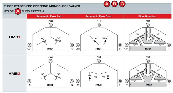
V1, V2 are the inside valves (A) (B) (C) are valves port sides
